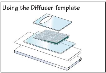
1. Build sandwich as illustrated. The Diffuser is used in place of one of the cutting pads. Never use Diffuser with more than one cutting pad!
