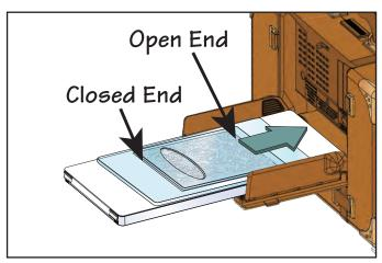
2. Align the Diffuser template with the closed end of the embossing folder. Insert into the machine open-end first as illustrated.
