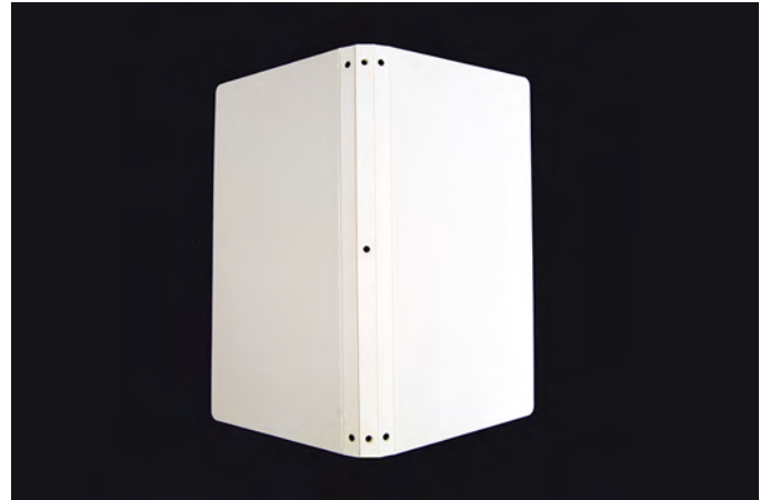
2. Overlap the center spine flaps of each side, and adhere them together.
